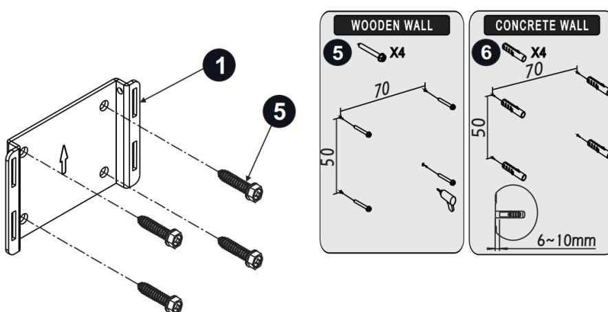
3. To mount the panel PC on the wall, align the wall mount bracket attached to the panel PC with the wall mount plate on the wall and slide the panel PC downwards to hang the bracket on the mount plate. Secure the panel PC in place by tightening screws in the wall mount bracket.
