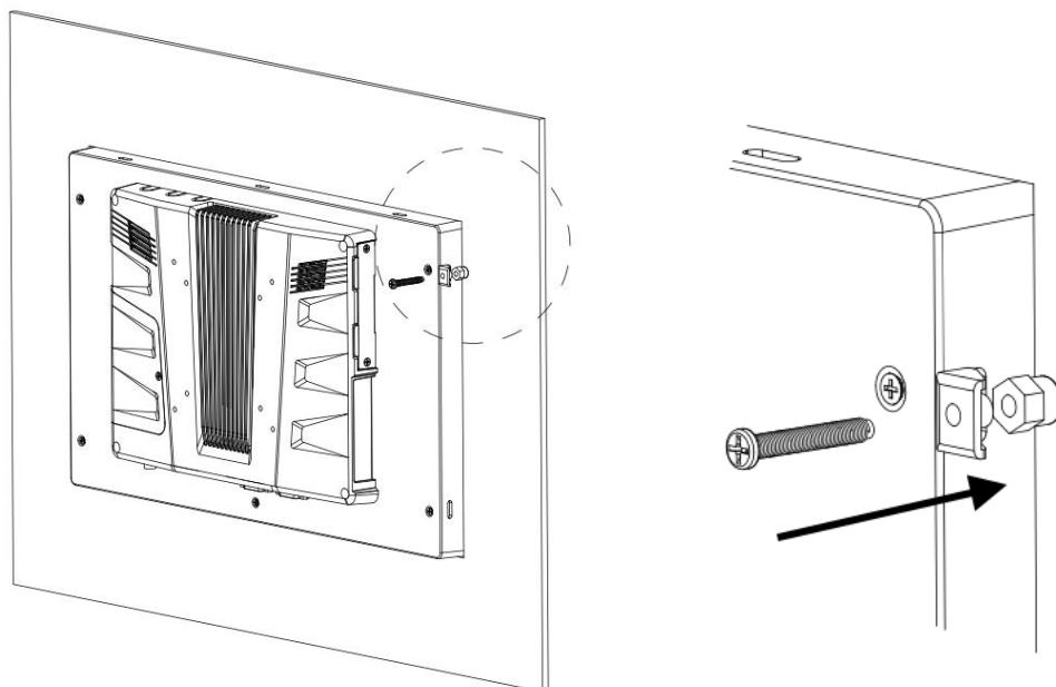
4. Tighten the screws to affix the panel PC in place, fasten all the hook bracket to ensure panel PC well fix at cabinet
