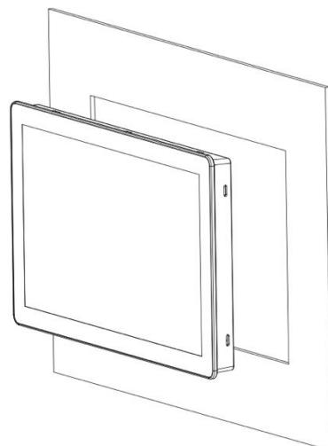
2. Install the panel PC in the cabinet and retrieve hook brackets from the accessory box
