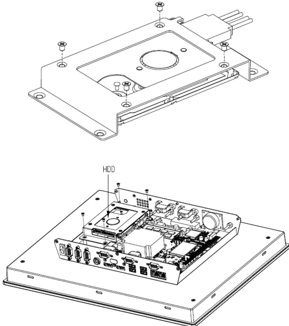
**Step 3.1 HDD Installation:** Insert the HDD into the Drive Bay and fasten 4 screws.
