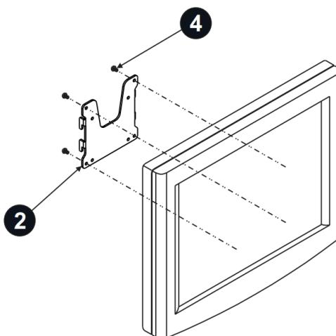
2. Select the location on the wall for the wall mount plate, secure the mount plate to the wall by inserting four M5 screws into pilot holes and tightening them.
