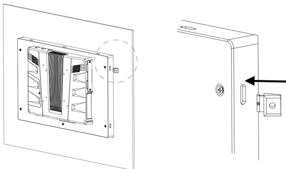
3. Insert the hook brackets into the holes following the direction of the arrows shown in below figure and hang the panel PC
