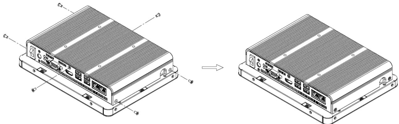
**Step 4.** Assemble the board and bottom chassis back as step 3 to step 1.
