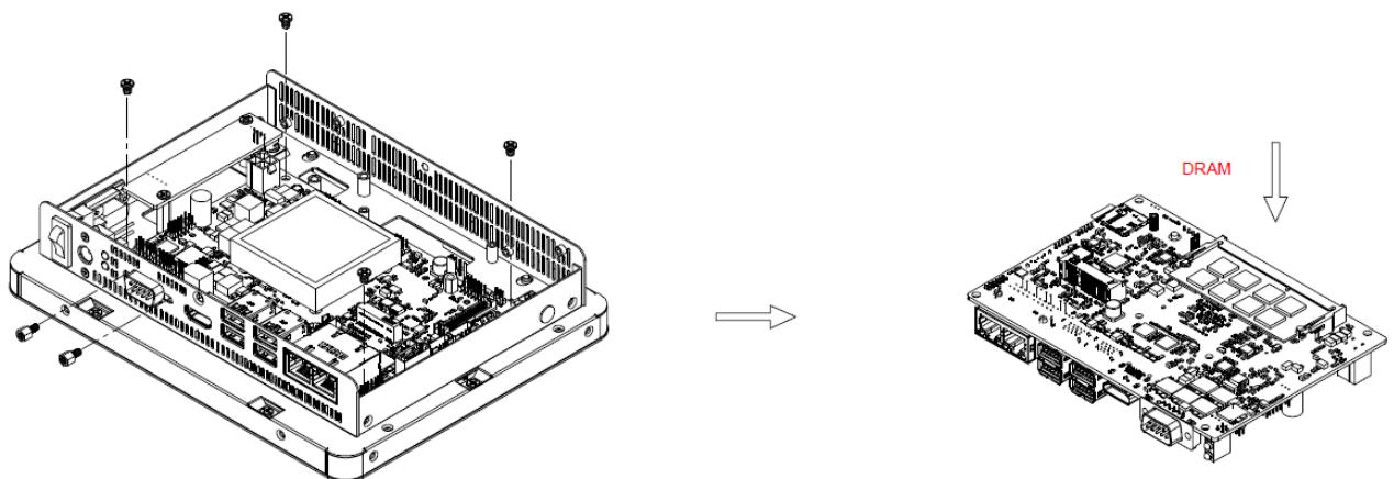
**Step 2.** Unlock 2 coppers from the rear I/O of VGA & COM ports.
