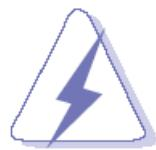
Class I Equipment. This equipment must be earthed. The power plug must be connected to a properly wired earth ground socket outlet. An improperly wired socket outlet could place hazardous voltages on accessible metal parts.
