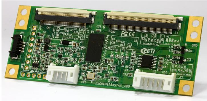
The EXC84H4254STAG is a projected capacitive (PCAP) touch screen controller that powered by EETI's high performance MCU EXC80H84. By integrating the advantages of self and mutual capacitance sensing technology, built-in high driving voltage transceiver and a powerful MCU, this controller incorporate most desired features to boost the noise immunity, and support high demand applications in most categories.
