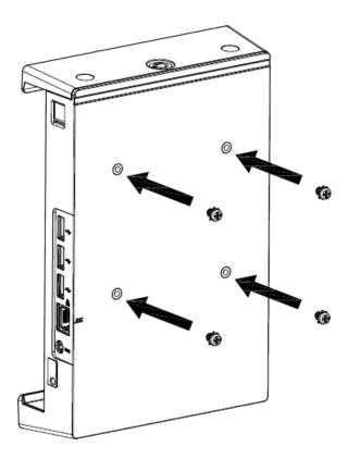
Step 1. Insert VESA into designated location and fasten with 4 screws to complete Installation.
