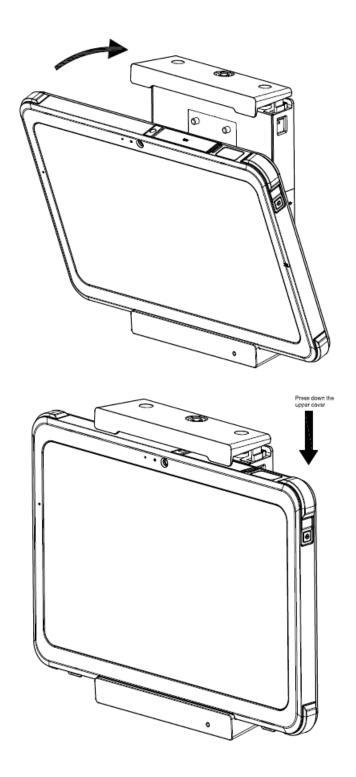
**Step 2.** Make sure the tablet is placed at the right position and press down the upper cover.
