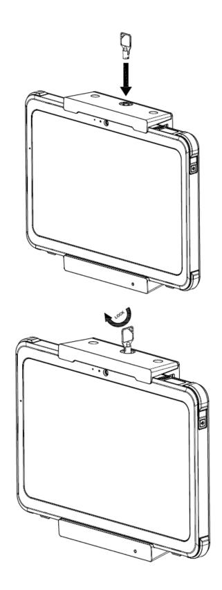
Step 3. Turn the key to lock in position. Make the texts on the image editable for localization Keep the key in a safe place. If you lose the key, contact the manufacturer.
