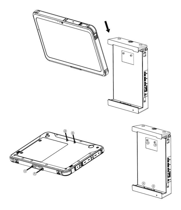
Fix the wall mounting station (with the tablet) to the toll stand or wall mounting racket. The mounting station connector complies with standard VESA interface.
