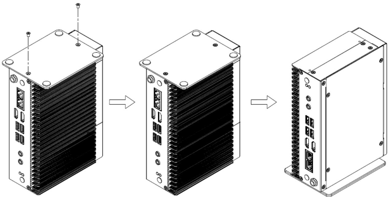
**Step1.** Fasten 2 screws on the side of the system to secure Stand.
