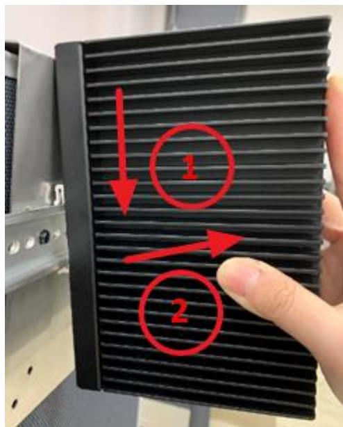
**Step4.** Push down the system (Press the Din-Rail) then remove the Din-Rail from the track.
