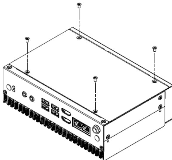
**Step1.** Remove 4 screws from the bottom of your system and take it off.
