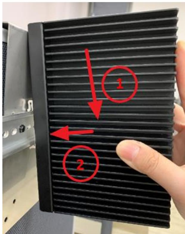
**Step1.** Slide the Din-rail into the track.
