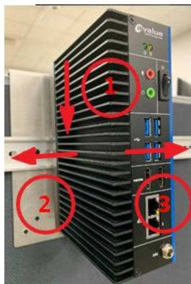
**Step3.** Push down the system (Press the Din-Rail) then move it right and left.
