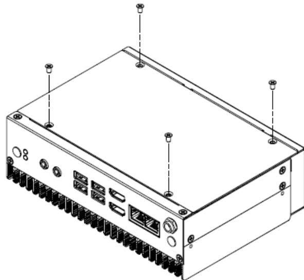
**Step3.** Place back the cover and fasten 4 screws back to complete
