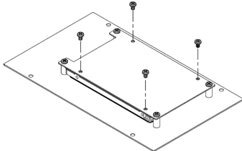
**Step2.** Fix HDD using the 4 screws in the Accessory Kit.
