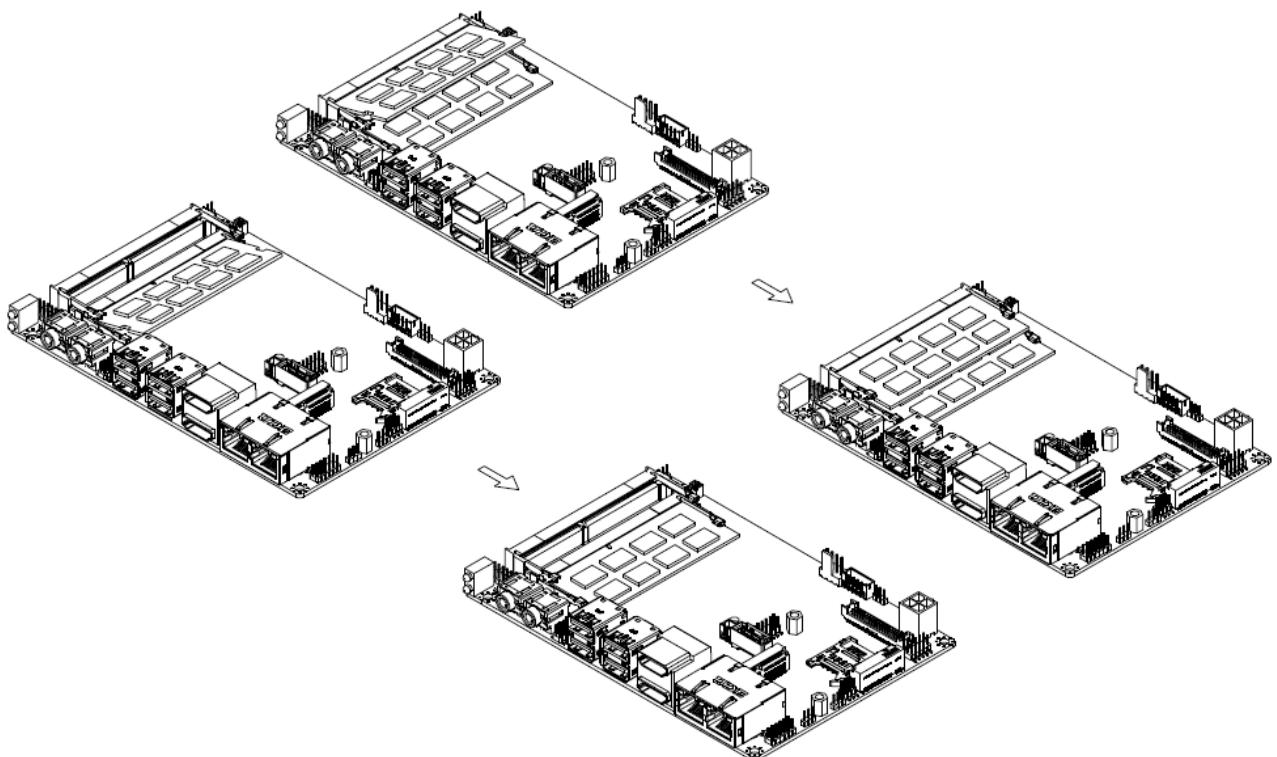
**Step4.** Properly install the memory modules and press until properly seated.
