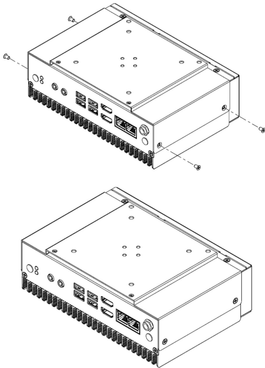
**Step1.** Remove 4 screws from the side.
