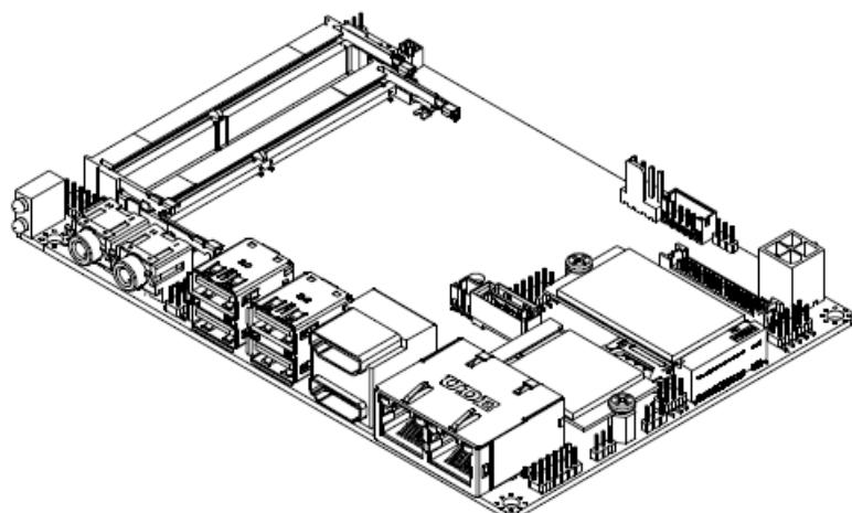
**Step1.** Insert M.2 B-Key card into designated locations and fasten with the screws to complete installation.
