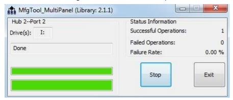
7) You can also get the information from Terminal (debug port→JUART1, baud rate set as **115200**) after flashing is finish
